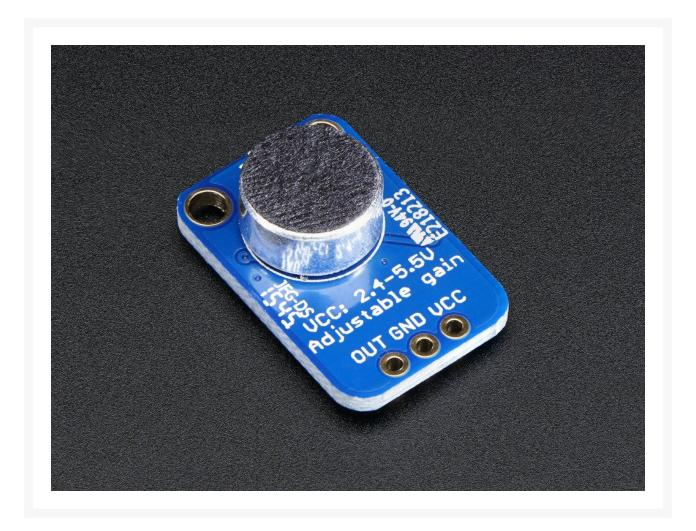
Add an ear to your project with this well-designed electret microphone amplifier. This fully assembled and tested board comes with a 20-20KHz electret microphone soldered on. For the amplification, we use the Maxim MAX4466, an opamp specifically designed for this delicate task! The amplifier has excellent power supply noise rejection, so this amplifier sounds really good and isn't nearly as noisy or scratchy as other mic amp breakouts we've tried!
